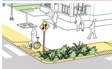
Curb Access for Wheelchair Users
