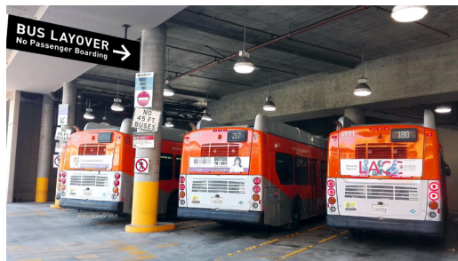
Bus Layover Designated area where buses can wait between trips so drivers can take breaks, and where vehicles can be fueled, charged, or cleaned.
